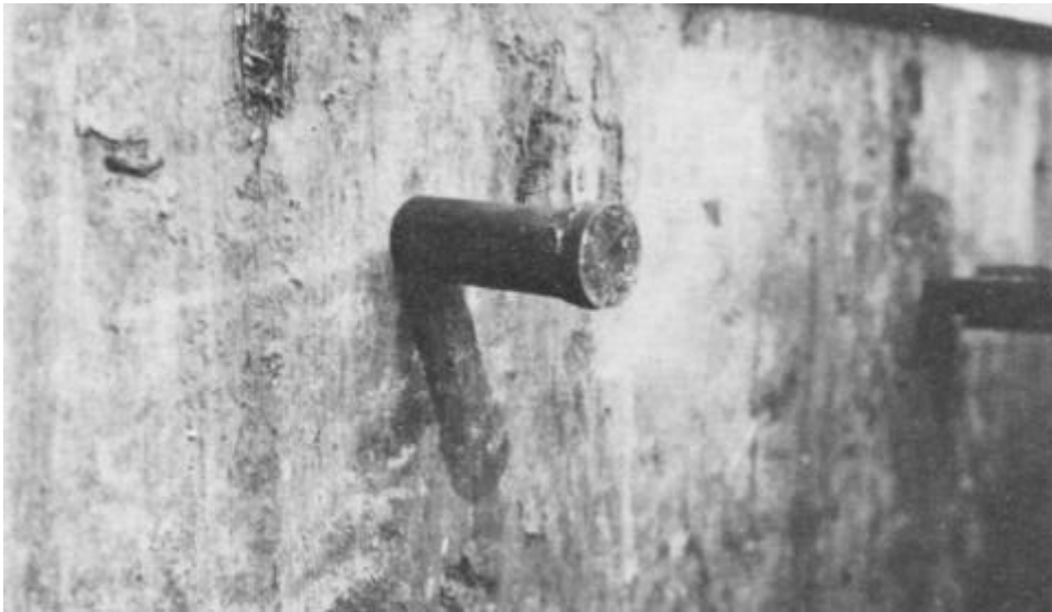
Figure C-11. Joint Meter Socket Screwed onto Plug (Courtesy of the Tennessee Valley Authority).
