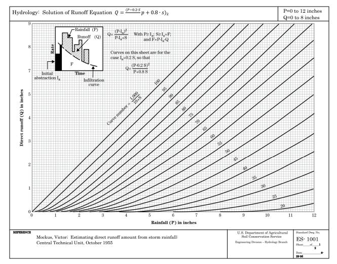
Figure 5-6. Solution for runoff equation
