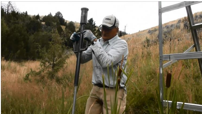
Photo 4: Installing Piezometer by Hand Auger
