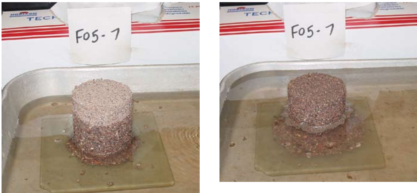
Figure 45B-3 Vaughan and Soares test on sample with poor self-healing characteristics. As sample is submersed, capillary stresses are reduced and sample should collapse. This sample does not collapse on wetting, demonstrating poor self-healing characteristics.
