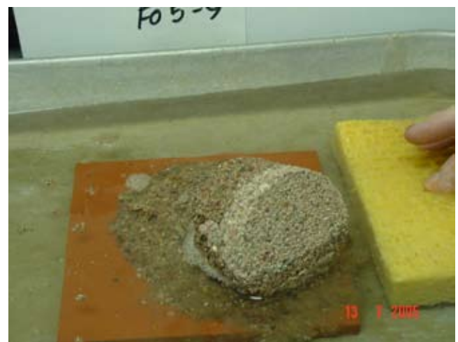
Figure 45B-4 Vaughan and Soares test on sample with good self-healing characteristics. As sample is submersed, capillary stresses are reduced and sample collapses quickly.
