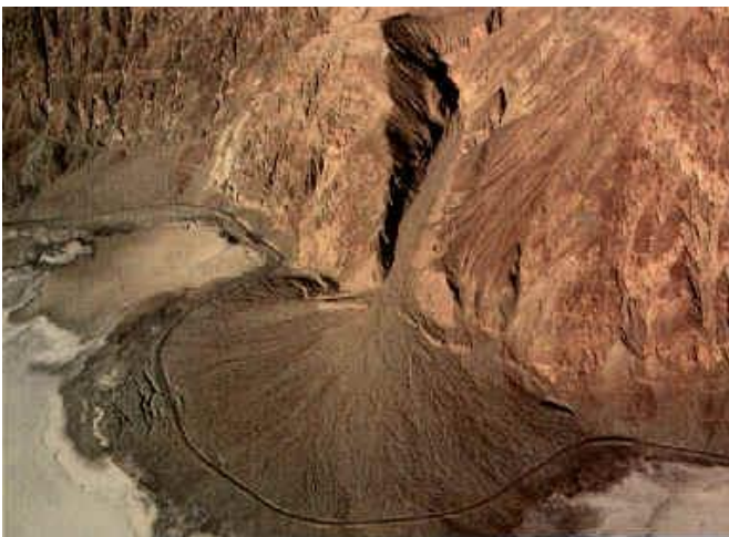
Figure 13 - Typical Alluvial Fan Deposit. Rock is Eroded from Above and Deposited Below as Soil.
