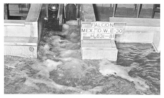
90-inch left valve fully open, discharging 2,400 c.f.s. Reservoir elevation 300, approx. Tail water elevation 181.2. FIGURE 96.—Falcon Dam: Mexican outlet works—model scale: 1:30.
