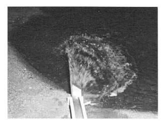
FIGURE 143. Dispersion-type flip bucket—Q=24,000 c.f.s.
