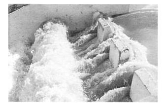
The second row of baffles is completely covered because of acceleration of flow between the first and second rows with a flow of 75 c.f.s. at top of baffled chute.
