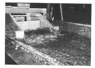
Hydraulic model discharging maximum capacity under similar conditions of head and tailwater.
