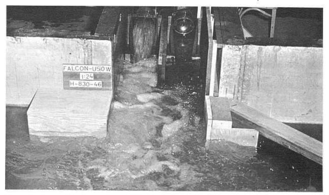
72-inch right valve fully open, discharging 1,600 c.f.s. Reservoir elevation 310, approx. Tail water elevation 180.5. FIGURE 98.—Falcon Dam: United States outlet works—model scale: 1:24.
