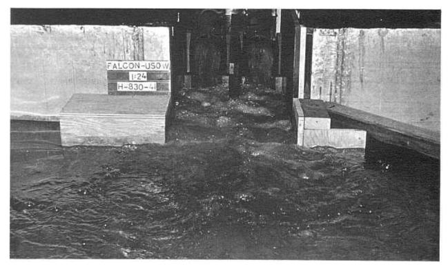
72-inch valves fully open, discharging 2,920 c.f.s. Reservoir elevation 310, approx. Tail water elevation 180.8. FIGURE 97.—Falcon Dam: United States outlet works—model scale: 1:24.
