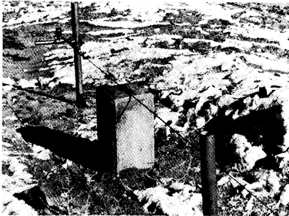
Figure 13-30. A tensioning device used with a tape for precise baseline measurements.—P557-D-58714
