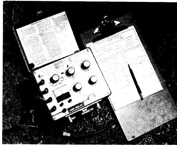
Figure 13-8. A special portable wheatstone bridge test set for reading strain meters.-C-8343-2
