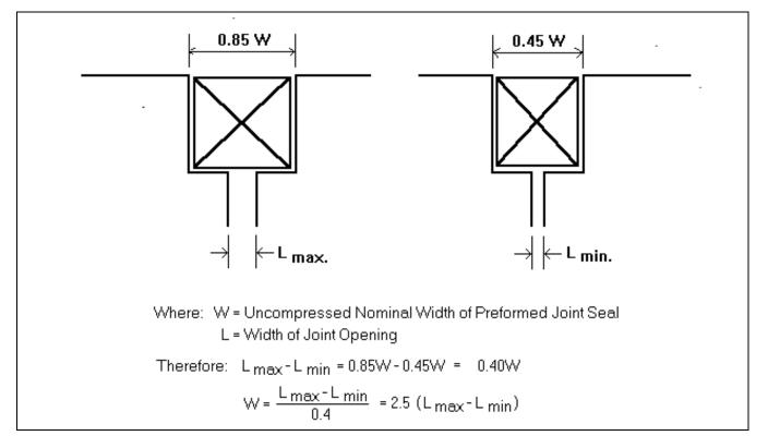
Figure 4-3. Determination of minimum size of compression seal
