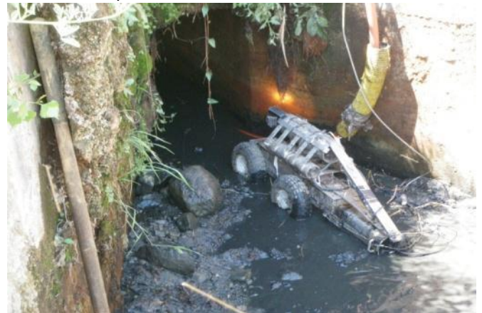
Photo 2: ROV entering a conduit for inspection.
