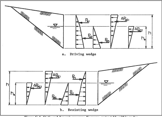
Figure G-4. Static and dynamic pressure diagrams, water table within wedge
