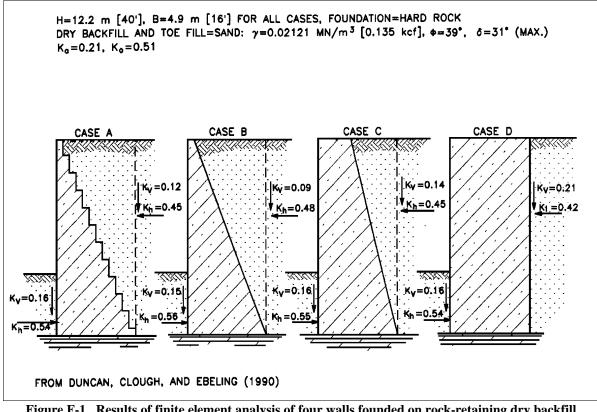
Figure F-1. Results of finite element analysis of four walls founded on rock-retaining dry backfill  $(K = value \text{ of } K_V \text{ shown in this figure})$
