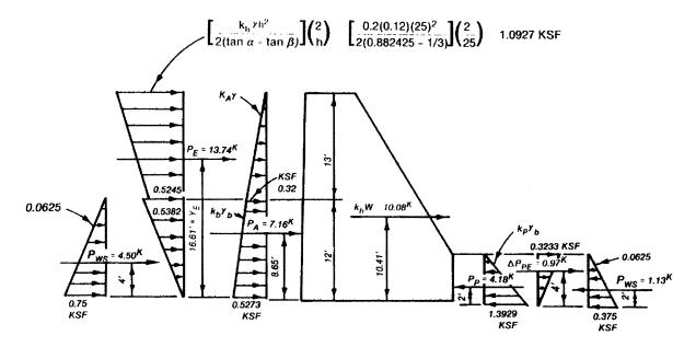
(1) Permissible simplification for dynamic earth pressure distribution—driving side. The discontinuity of this pressure diagram, at the water table, may be eliminated by considering that the soil weight above and below water is equal to the moist weight. The difference is not significant. In this case, the difference in forces is -0.58% and difference in dimension,  $Y_E$ , is +0.36%.
