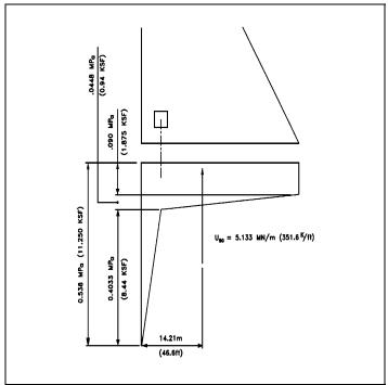
Figure D-9 Uplift with 90 percent drain efficiency
