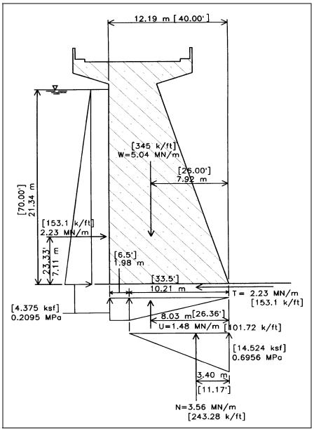
Figure D-11. Stability without tensioned structural anchors
