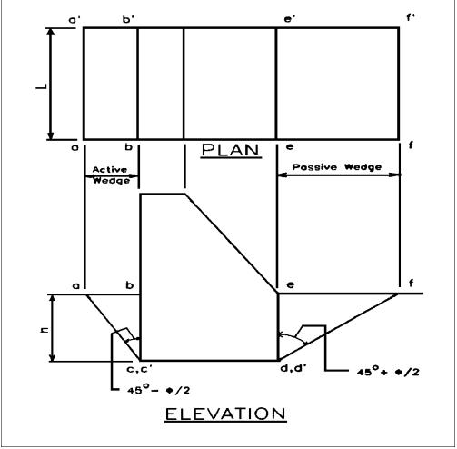
Figure 6-1. End effects on short wall
