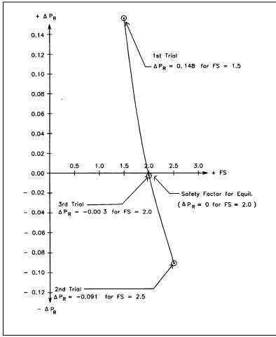
Figure D-4 Graphical solution for safety factor
