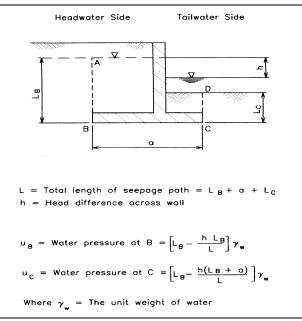
Figure C-1 Line-of-seepage method for water pressures
