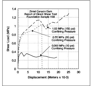
Figure D-14. Direct shear test for moderately to intensely weathered basalt
