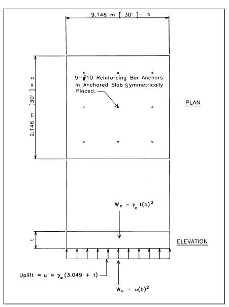
Figure D-17 Anchored spillway slab
