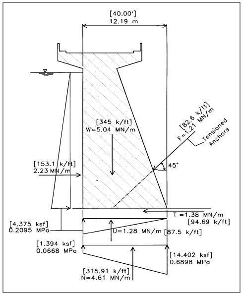
Figure D-12. Stability with tensioned structural anchors
