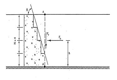
(b) Mass concrete wall with a stepped backside
