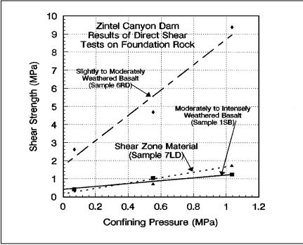
Figure D-16 Shear strength versus confining pressure
