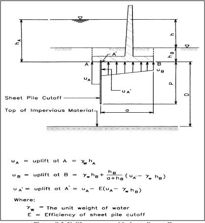
Figure C-3 Uplift pressures with sheet pile cutoff
