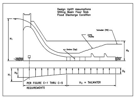
Figure C-5 Stilling basin with discharge condition
