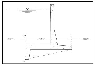
Figure C-2 Seepage path for wall with key
