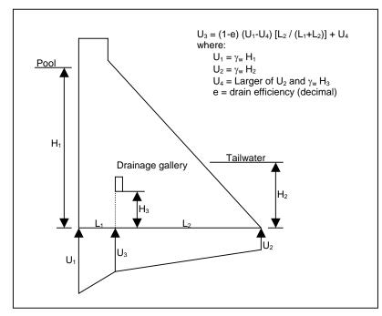
Figure C-4 Uplift distribution with foundation drains
