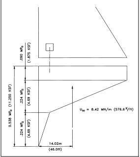
Figure D-8 Uplift with 50 percent drain efficiency (Resultant in middle 1/3 of base)
