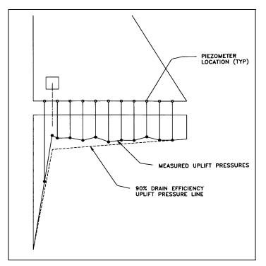
Figure D-10 Measured uplift versus 90% drain efficiency
