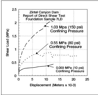
Figure D-15 Direct-shear test for shear zone material
