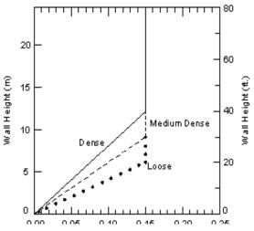
Figure F-3 Design values of K<sub>v</sub> for gravity walls founded on rock, with a vertical face against the backfill
