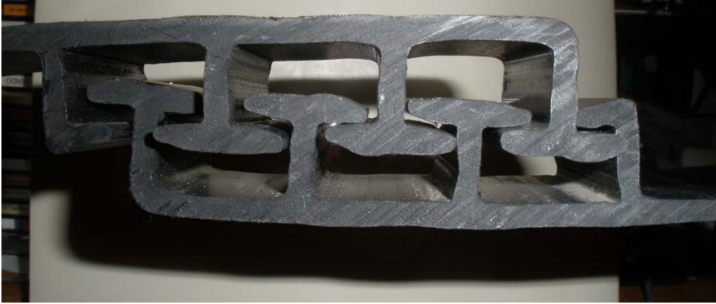
Figure 20.3.4-2. Geomembrane interlock (top view).
