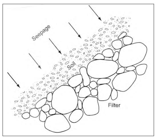
Figure 1-1. Schematic demonstrating the manner in which a properly designed filter prevents the movement of base soils by seepage forces at the discharge face. The filter supports the discharge face with closely spaced contact points as compaction melds the two zones together such that bridging between the contact points prevents any movement of base soil particles into the filter. At the same time, the filter is sufficiently coarse to allow seepage water to escape freely.
