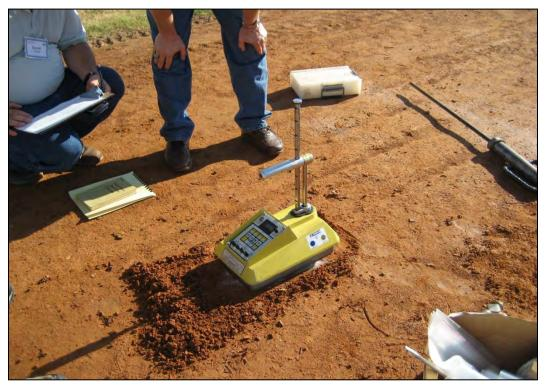
Figure 7-29. Typical nuclear moisture-density meter.
