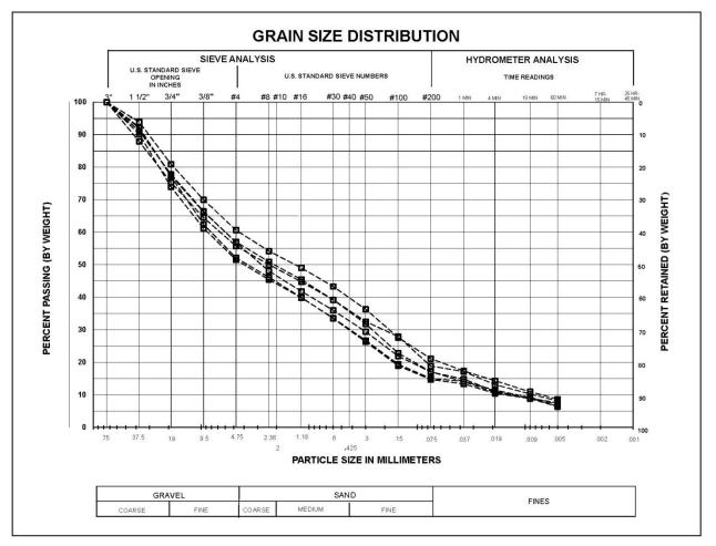
Figure 5-11. Existing embankment dam core gradations before re-grading.
