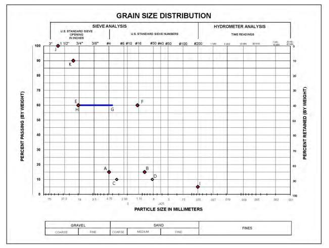
Figure 5-17. Filter Control Points for Interface 2.
