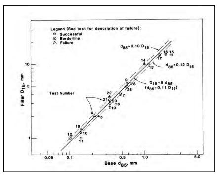
Figure L-10-1.—Relationship between  $D_{15}$  and  $d_{85}$  in initial SCS filter tests on sands and gravels.
