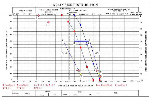
Figure G-2. Example particle retention filter gradation.
