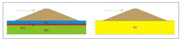
Figure A-5. Geologic cross section of three alluvial deposits that is simplified to one unit due to material uniformity.
