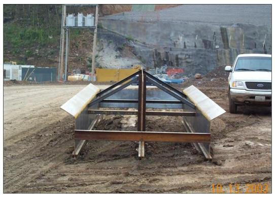
Figure 7-15. Double-bin spreader box.
