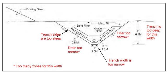
Figure E-11. Poor toe drain design elements.
