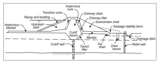
Figure 2-3. Typical embankment dam design elements found in a central core design.
