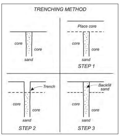
Figure 7-4. Steps for trenching method.
