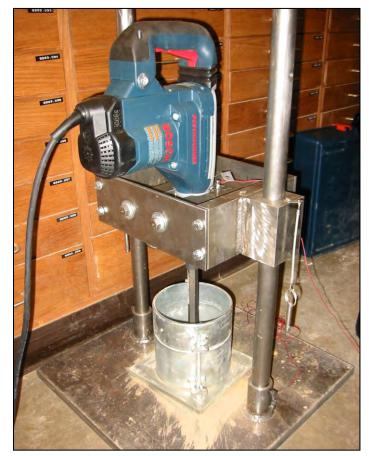
Figure 7-31. Vibratory hammer used to obtain a reference density value for filter materials. (Photo courtesy of Dr. Vincent Drnevich)
