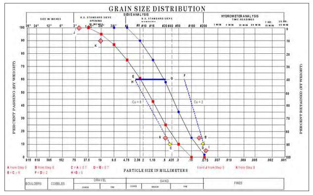
Figure G-4. Example transition zone gradation.
