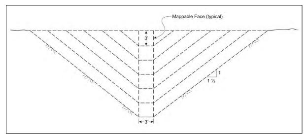
Figure 6-8. Exploration trench excavation sequence.
