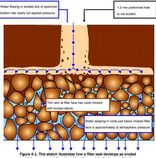
particles are carried from the sides of a crack in the base soil to the filter face. Eroded particles accumulate and create a filter seal that effectively blocks further flow and subsequent particle movement (after Sherard, 1984).
