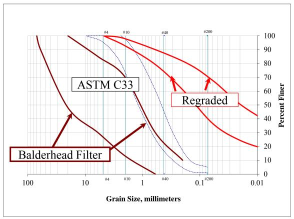
Figure L-9-1.—Re-graded core zone from Balderhead case history.
