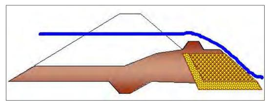
Figure E-1. Cross-section of embankment at time of overtopping.
