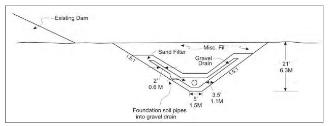
Figure E-9. Piping of foundation soil into gravel drain.
