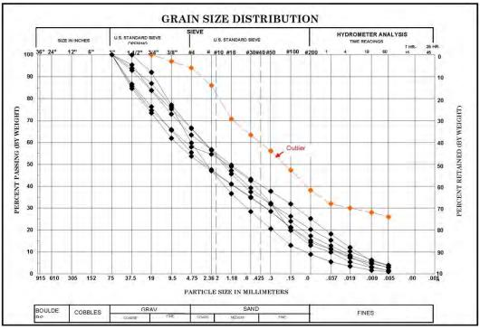
Figure A-10. Gradation test samples including an outlier.
