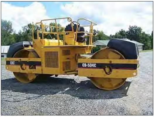
Figure 7-21. Double-drum vibratory roller.
