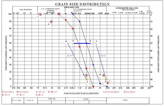
Figure G-3. Example drainage filter gradation.
