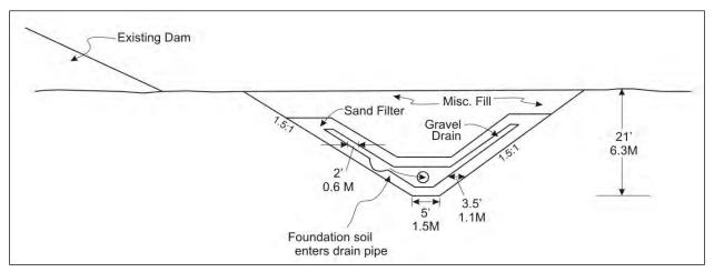
Figure E-10. Foundation soil passes through gravel drain and enters drain pipe.
