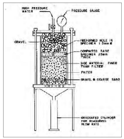
Figure F-1. Filter test details (schematic).
