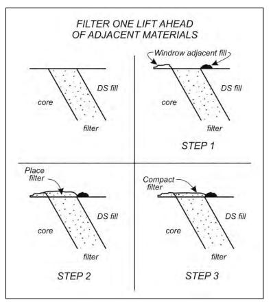
Figure 7-2. Steps in maintaining a chimney one lift ahead of impervious core.
