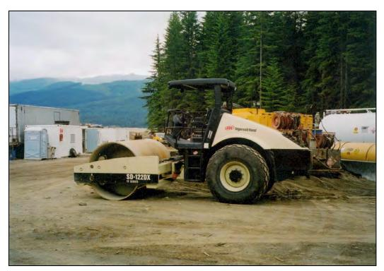
Figure 7-22. Single-drum vibratory roller.
