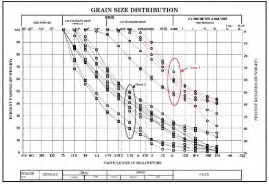
Figure A-7. Gradation plot of alluvial fan material indicating two distinct units.
