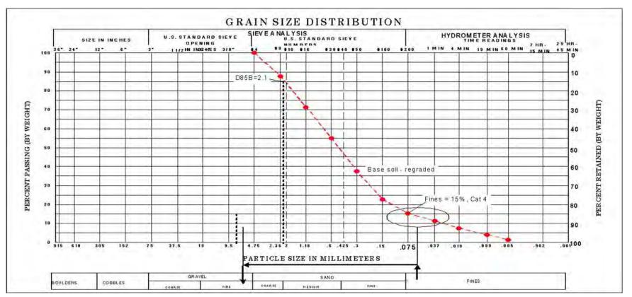
Figure 5-5. Illustrative re-graded base soil curve.
