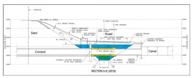
Figure 3-2. Typical filter addition around a conduit near the downstream toe of a dam.
