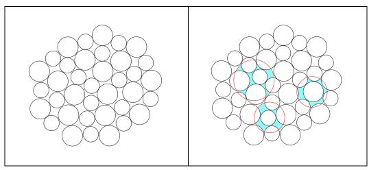
Figure 6-5. The illustration on the left shows idealized spheres of two sizes and resulting void space between the spheres. For the illustration on the right, three larger spheres (red) are overlain on the original illustration. This demonstrates how the larger spheres will replace once available void space, highlighted in blue.
