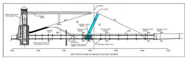
Figure 3-1. Typical filter addition around a conduit near the centerline of a dam enlargement.
