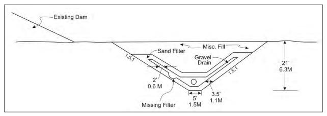
Figure E-8. Area of possible filter damage.
