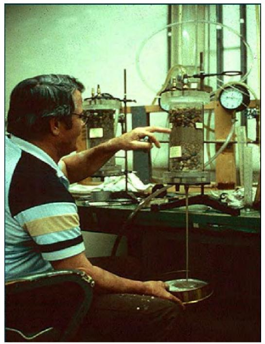
6. A plastic liner may be used in the mold to ensure separation of the sand from the mold when disassembled.
