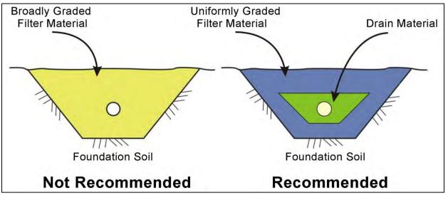
Figure 2-12. Typical one-stage (left) and two-stage (right) toe drains in a trapezoidal trench.
