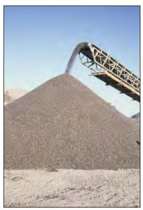
Figure 7-7. Conical stockpile.
