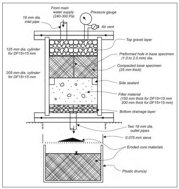
Figure 4-3. CEF test apparatus.
