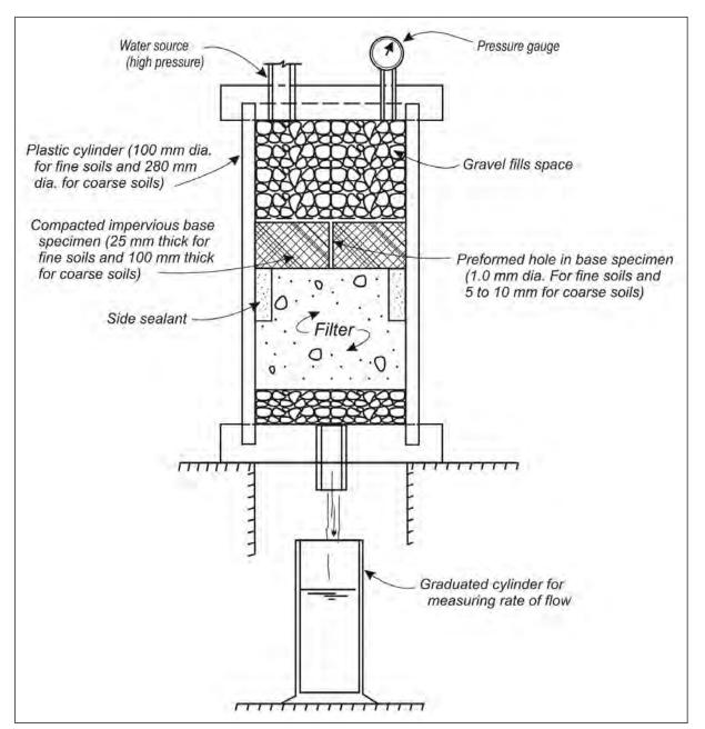
Figure 4-2. NEF Test apparatus.
