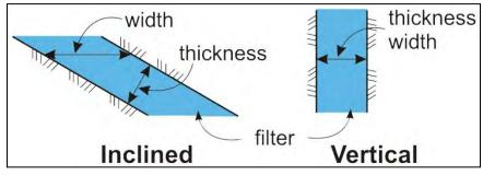
Figure 6-2. Definition of filter width and thickness.
