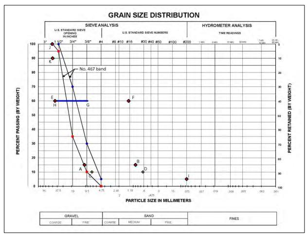
Figure 5-18. Gradation for ATSM D448 No. 467 material plotted with modified control points for Interface 2 (allow for particle rearrangement).
