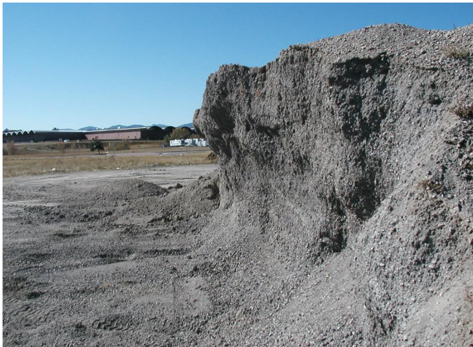
Figure 5.8.4-1. Sand and gravel stockpile (recycled concrete) that indicates fines or binding agents are present due to verticality and overhang seen in the slope.
