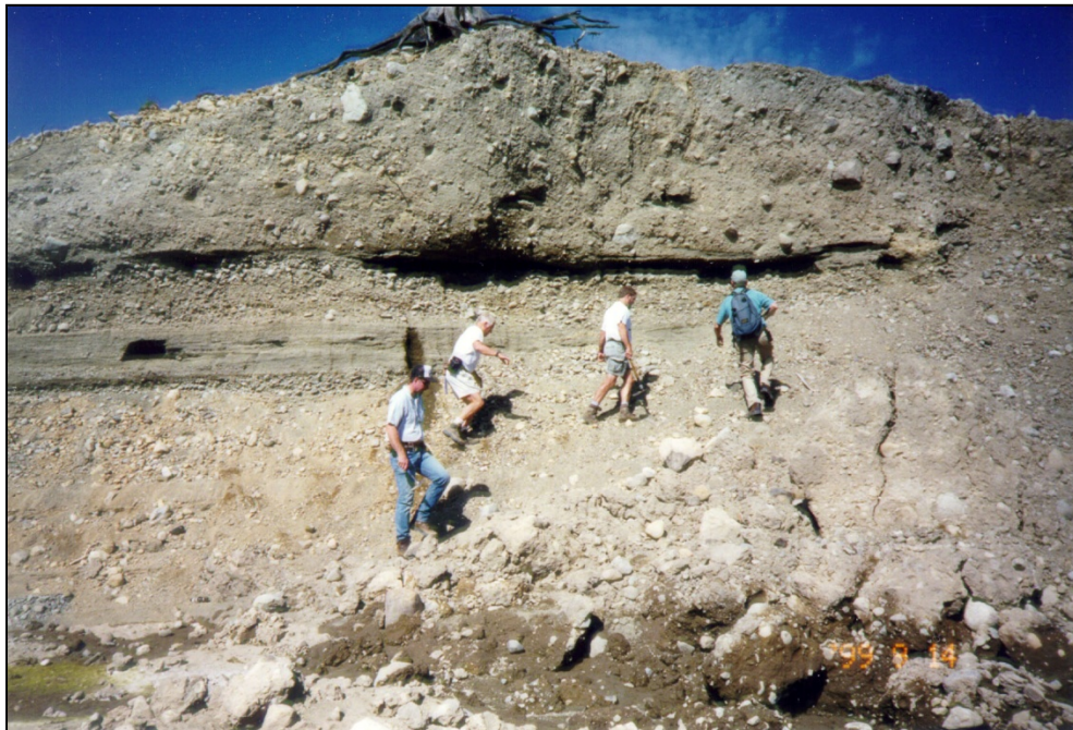
Figure 5.7.1-1. Exposed moraine cross section showing till overlying glacial outwash. Such exposures provide an opportunity to obtain geologic information by observation.
