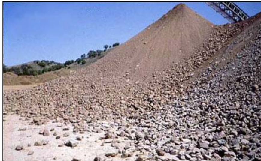
Figure 5.8.3.2-1. Segregation at high stockpile of broadly graded material. This photograph is an example of roll down segregation, and the shown material would not be acceptable for use as a filter (photo courtesy of A. Breitenbach).
