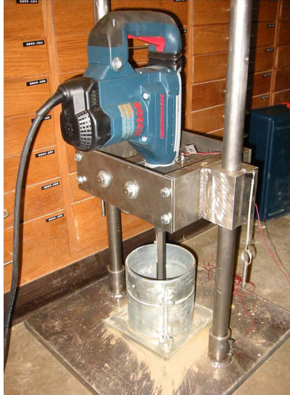
Figure 5.8.7.2.7-1. Vibratory hammer used to obtain a reference density value for filter materials. (Photo courtesy of Dr. Vincent Drnevich.)
