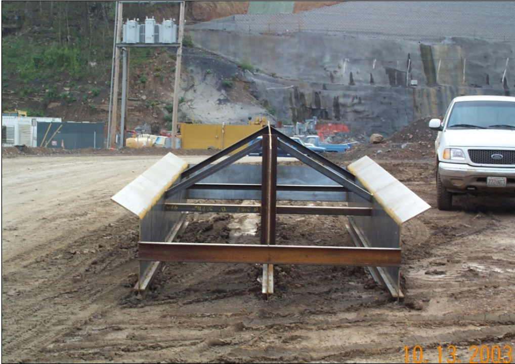
Figure 5.8.2.5.2-2. Double-bin spreader box.
