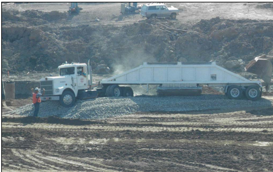
Figure 5.8.2.4-2. Articulated bottom-dump truck. The photo illustrates difficulty that can arise when the truck dumps too quickly for the speed of the truck. The trailer will then hang up and require assistance from other equipment.
