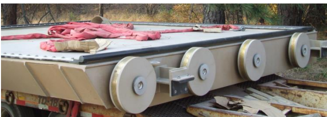
Photo 3: Fixed Wheel Gate
