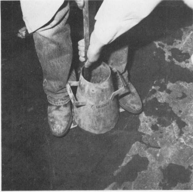
(a) Rodding and filling cone using three separate layers of concrete.
