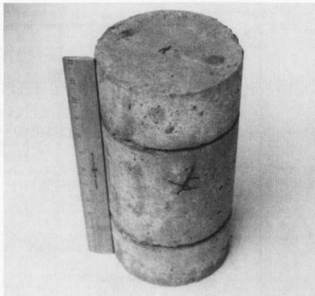
Figure 5. - A cast concrete permeability cylinder showing grooves formed by the collars shown on figure 4.
