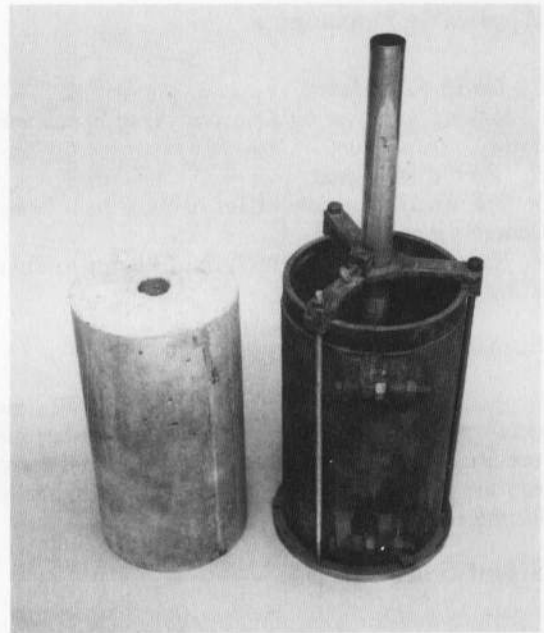
Figure 3. - Mold and 8- by 16-inch (203- by 406-mm) cylinder with a 1.5-inch (38-mm) hole through the center.
