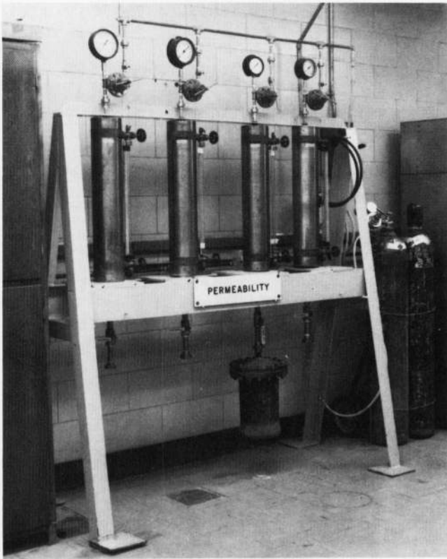
Figure 2. – View of permeability apparatus showing compressed-air cylinder (right) and testing units.
