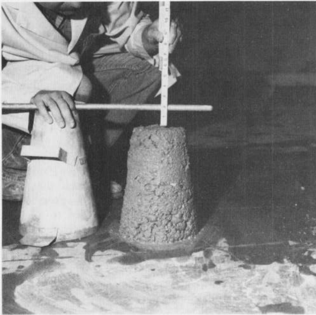
(c) Measuring the slump after subsidence.
