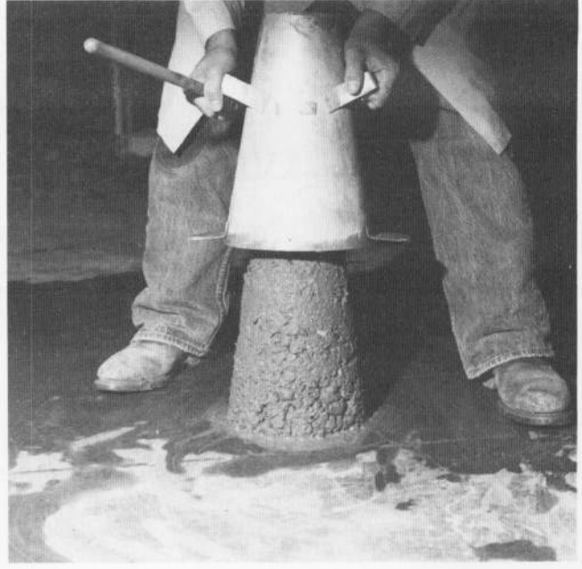
(b) Slow, steady, vertical removal of mold.
