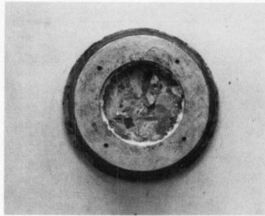
Figure 8. - View of bottom of specimen container showing method of applying plaster of Paris to container flange.
