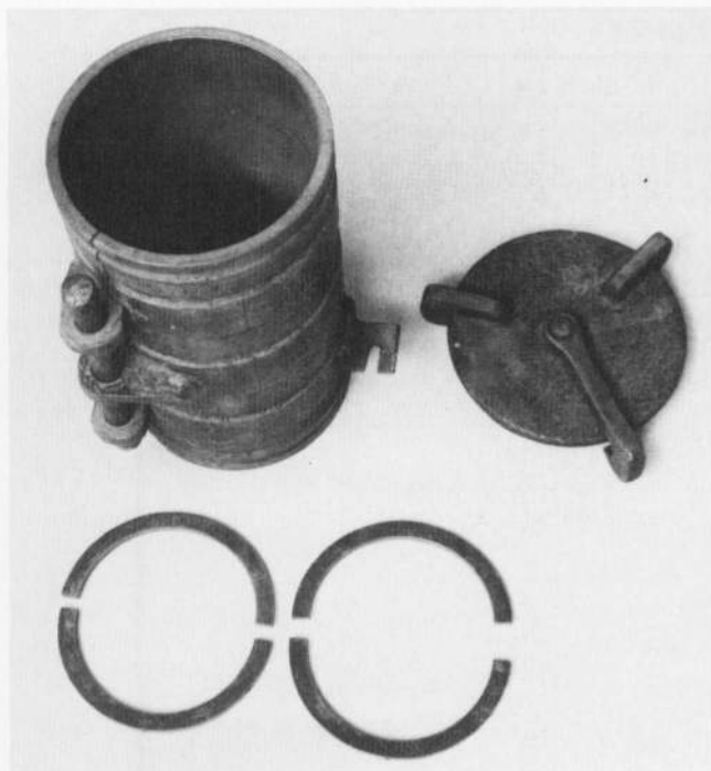
Figure 4. - A 6- by 12-inch (152- by 305-mm) cylinder mold with collars (rings) that provide grooves in the concrete.
