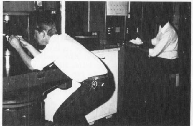
Figure 6. - Calibrating a testing machine in compression.
