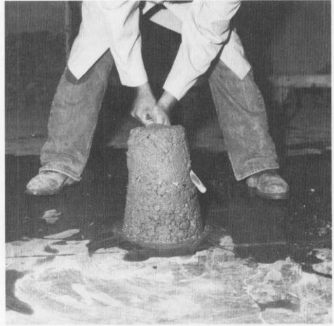
(d) Tapping the concrete to observe the plasticity.
