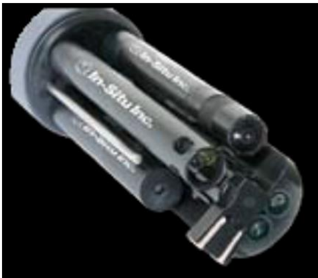
Figure 21.8.10-8. Multi-parameter automated probe with interchangeable sensor arrays (reprinted with permission from In-Situ Co.).
