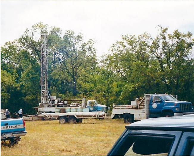
(b) 2-ton flatbed rig
