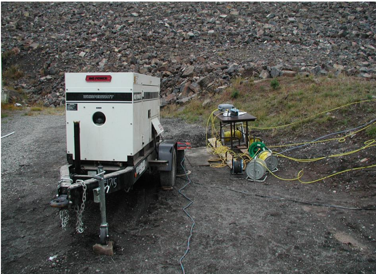
Figure 21.8.10-9. Typical aquifer test setup. Data logger is connected to pressure transducers in a pumping well and observation wells and is set up near the generator that is powering the submersible pump. This allows the WR&C specialist to monitor the progress of the aquifer test and power supply (Grassy Lake Dam, Wyoming, photo by W. Robert Talbot).
