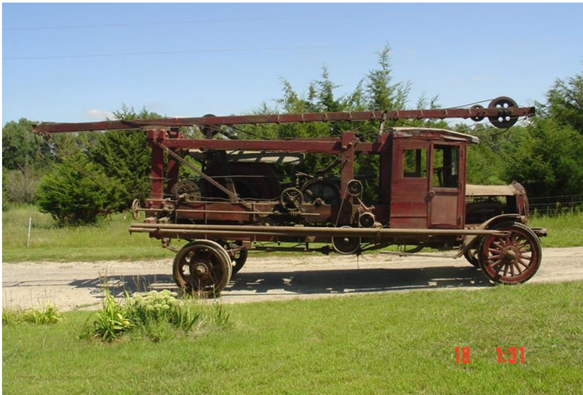
Figure 21.9.2-4. State-of-the-art cable tool rig, circa 1935 (reprinted with permission from Johnson Screens, Inc.).
