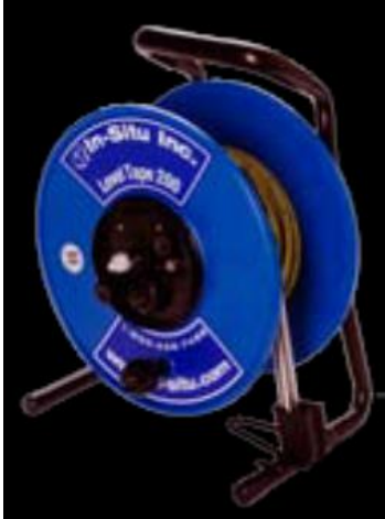
Figure 21.8.10-4. Electronic water level sensor (reprinted with permission from In-Situ Co.).
