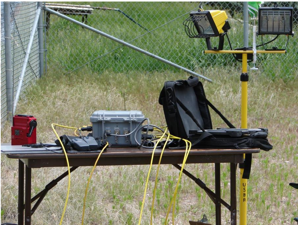
Figure 21.8.10-6. In-Situ Hermit 3000® data logger and rugged field laptop. Data logger is connected to dedicated pressure transducers via the yellow, vented cables. Data is downloaded from the data logger to the laptop every 8 hours in case of data logger failure. Light tower is for night-time monitoring of the aquifer test (Red Willow Dam, Nebraska, photo by W. Robert Talbot).
