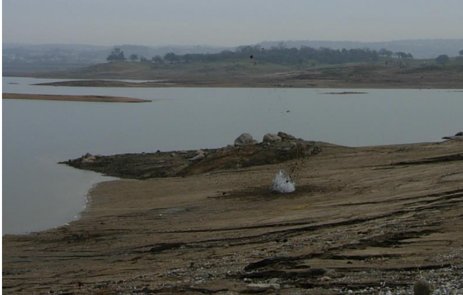
Figure A-9. Explosive seismic source for SRT survey. (Photo by Rich Markiewicz, Reclamation)
