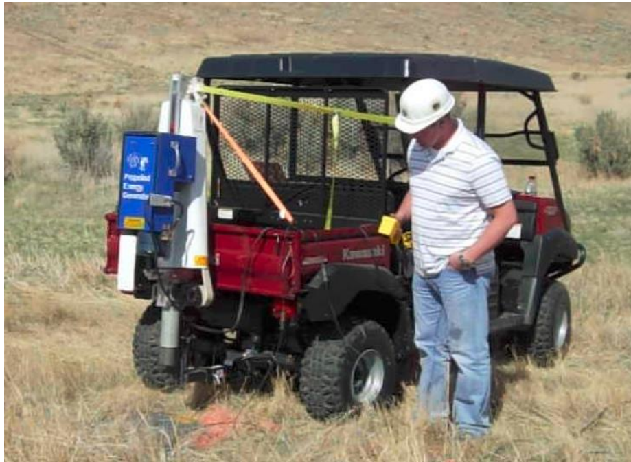
Figure A-8. Weight drop seismic source mounted on the back of a utility vehicle. The weight drop piston is accelerated by means of large elastic straps, and impacts upon a metal ground plate. (Photo by Rich Markiewicz, Reclamation)
