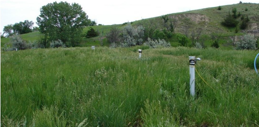
Figure 21.9.4-2. A line of four observation wells in a field. They are being used to monitor an aquifer test, so all of their locking caps have been removed and temporary pressure probes installed. The depth of the probes are secured in place with loops of extra transducer cabling taped to the top of the well's surface casing as seen on the closest well (the closest well has extra yellow cabling taped to the top of the surface casing with electrical tape (Red Willow Dam, Nebraska, photo by W. Robert Talbot).
