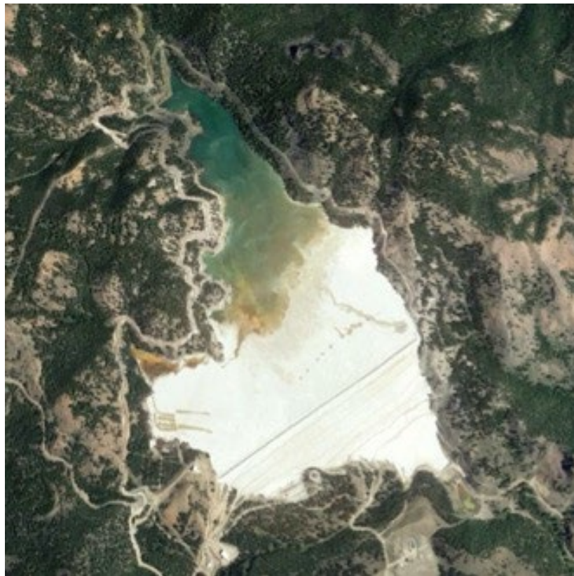
Figure III-3. Tailings dam at hard rock mine constructed by the centerline method (Google Earth, 2016)
