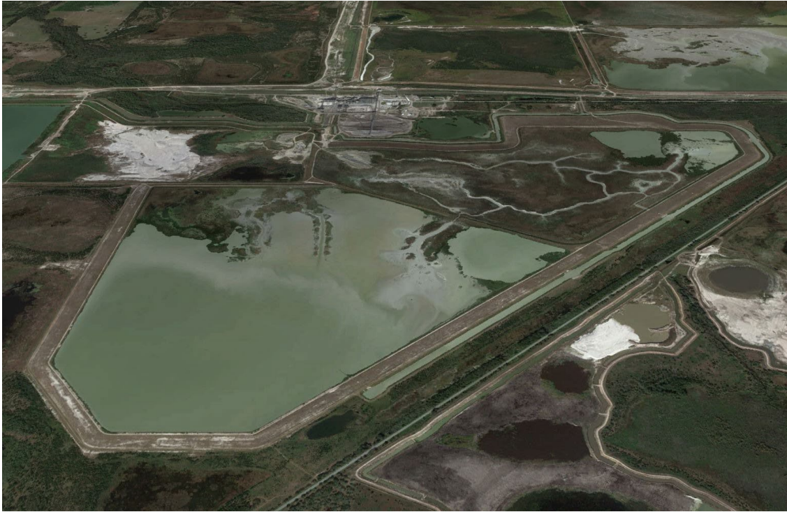
Figure III-6. Sand tailings dam for waste clay settling pond at soft rock mine (Google Earth, 2016)
