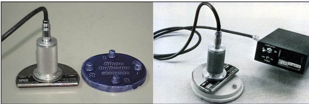
Figure 11.6.2.4-1. Portable tiltmeter and mating plate on the left, ready to collect data using the readout device on the right.
