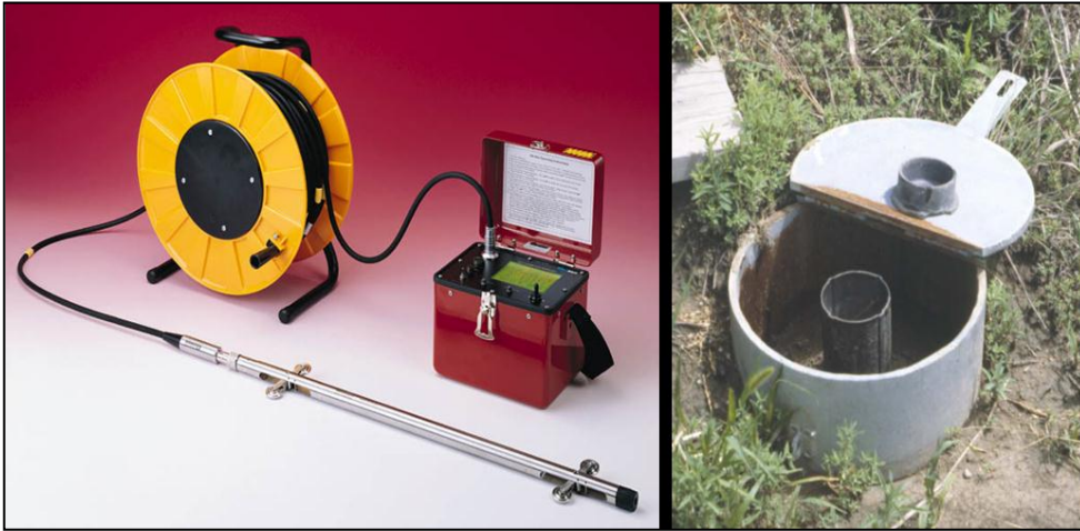
Figure 11.6.2.3.2-1. Left: An inclination probe, inclinometer cable, and an inclinometer readout unit. Right: Top of a typical installation as might be seen at a dam site.
