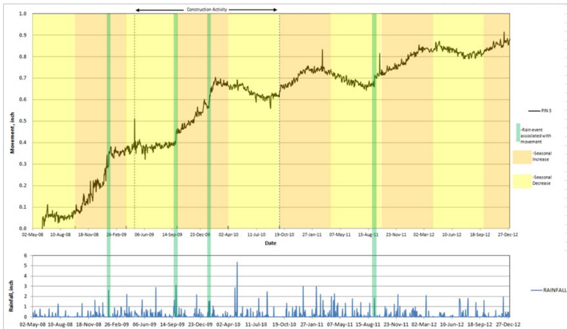
Figure 9.17. Crack Cumulative Displacement: 2008–2012
