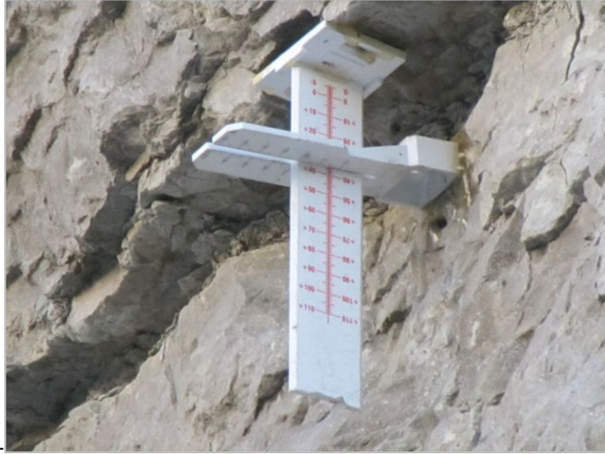
Figure 5.19. Visually Read Crackmeter with Slit Ruler
