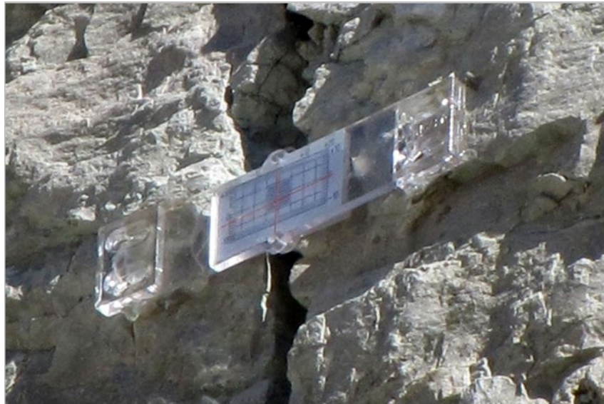
Figure 5.18. Visually Read Crackmeter with Cross-Hairs
